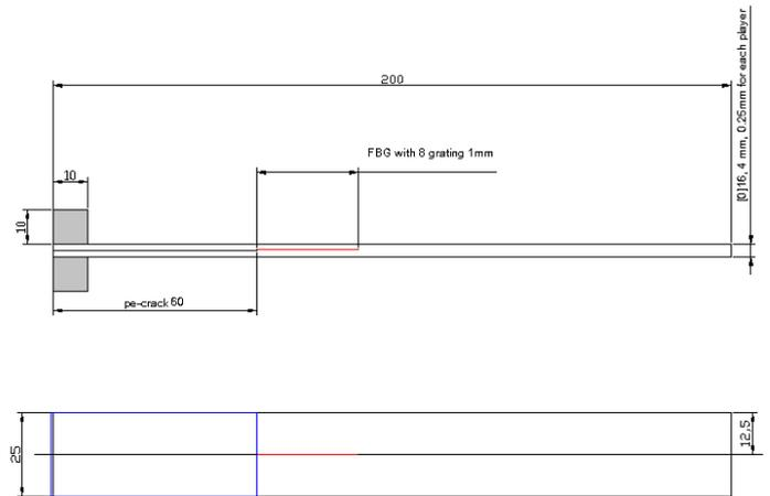
Fig. 5 DCB specimen dimensions used in numerical model.
