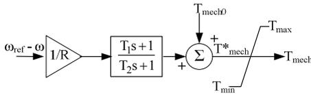
Fig. 4 Turbine governor model used for simple hydro generator: Model 2
