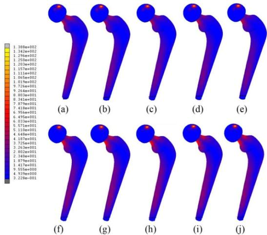
Fig. 10 The stress distribution on hip prosthesis under dynamic climbing stair at every 10 second: (a) 10, (b) 20, (c) 30, (d) 40, (e) 50, (f) 60, (g) 70, (h) 80, (i) 90 and (j) 100 second
