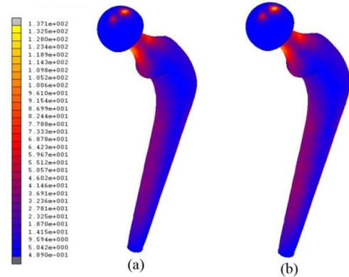
Fig. 8 The stress distribution on hip prosthesis under: (a) static walking and (b) static climbing stair condition
