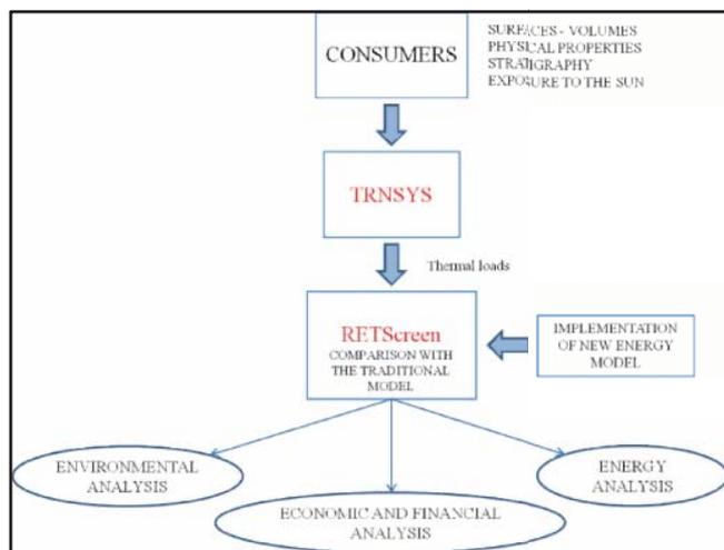
Fig. 5 Logic of the new design methodology
