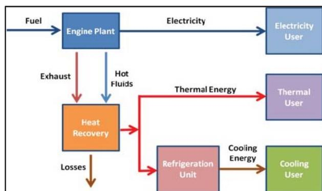
Fig. 3 Block diagram of the trigenerative plant
