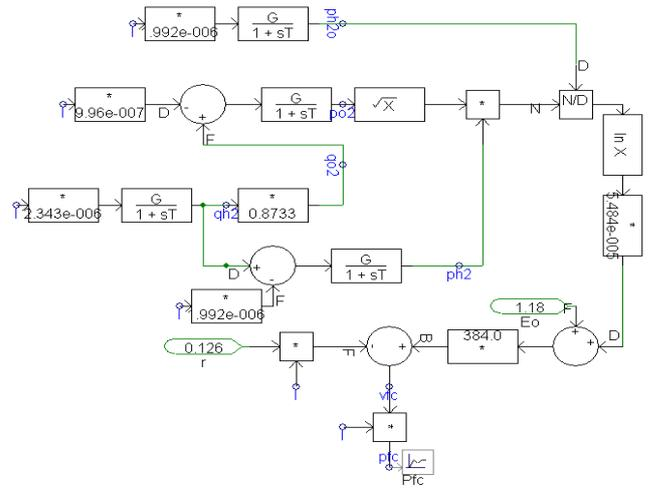
Fig. 4 PSCAD/EMTDC implementation of SOFC
