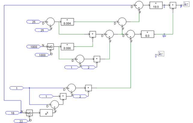
Fig. 5 PSCAD/EMTDC implementation of photovoltaic
