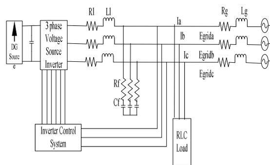
Fig. 3 Inverter control system for each distributed generation
