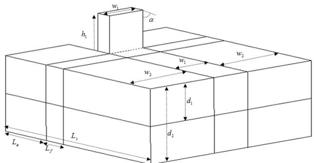
Fig. 2 Geometrical parameters of the FE model
