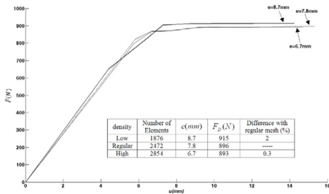
Fig. 6 Effect of e (and the mesh density) on the average draft force
