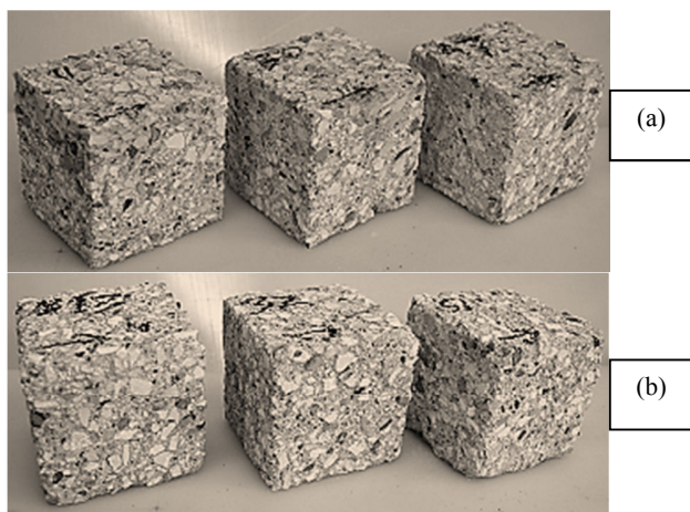
Fig. 5 Cube samples 11, 30 and 47 (left to right) after 42 days immersion into 0.5 pH sulphuric acid solution and temperatures of 10°C, 20°C and 30°C, respectively (a) and cube samples 13, 32 and 51 (left to right) after 56 days immersion into 0.5 pH sulphuric acid solution and temperatures of 10°C, 20°C and 30°C, respectively (b)
