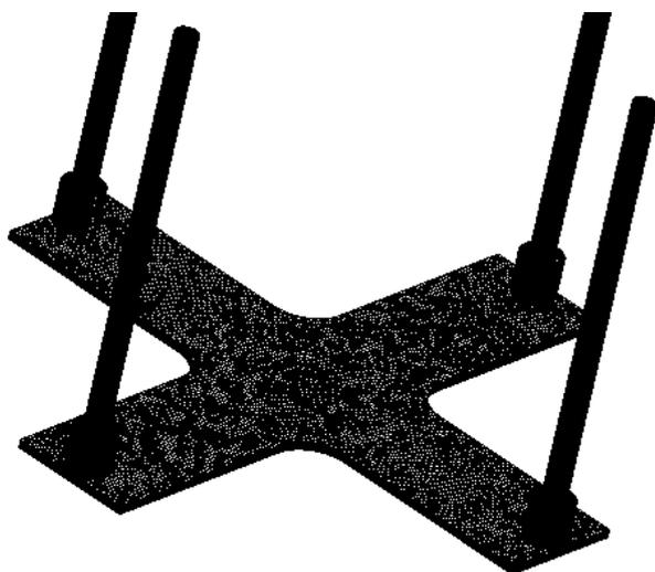
Fig. 4 Numerical grids of a cross-shaped micro channel at angle of 90° in a stereogram view
