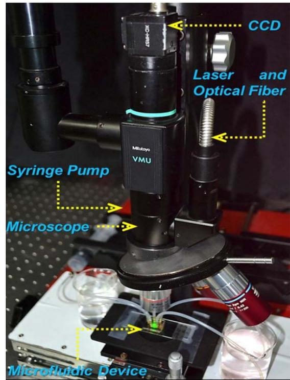
Fig. 3 Picture of the micro-flow visualization system
