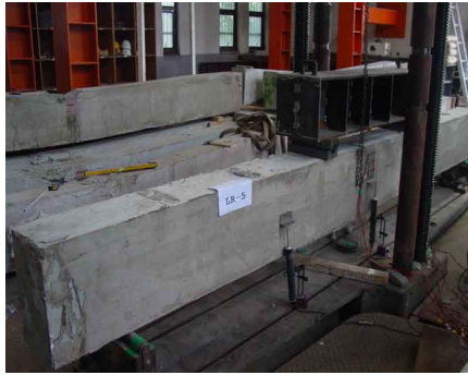
Fig. 6 Four point loading test set up
