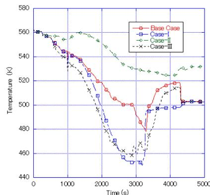
Fig. 8 Cold-Leg Fluid Temperatures in Broken Loop
