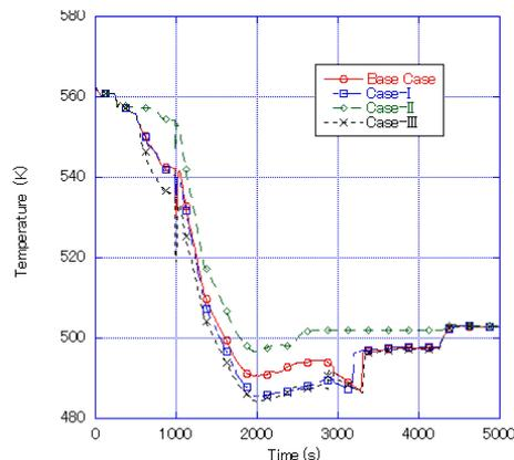
Fig. 7 Cold-Leg Fluid Temperatures in Intact Loop
