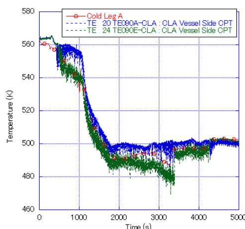
Fig. 4 Cold-Leg Fluid Temperatures in Intact Loop
