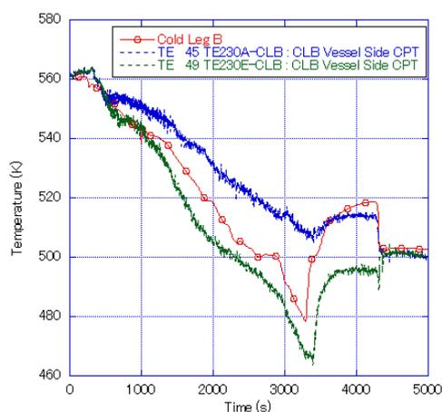
Fig. 5 Cold-Leg Fluid Temperatures in Broken Loop
