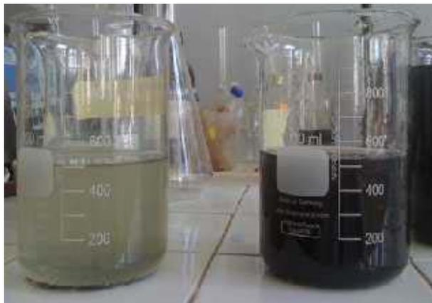
Fig. 3 Secondary wastewater clarified by *Moringa oleifera*
