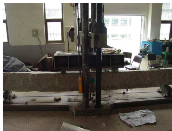
Fig. 5 Four-point loading test of rehabilitated beam
