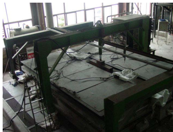
Fig. 4 The horizontal heating furnace for fire test
