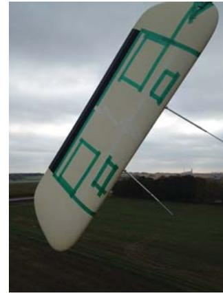
Fig. 2. The wing section with the flap mounted on the rotating rig test stand
