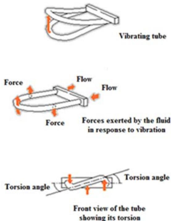
Fig. 7 Coriolis Measure
