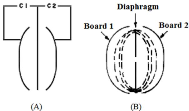
Fig. 4 Model of Capacitors in Cell Capacitive
