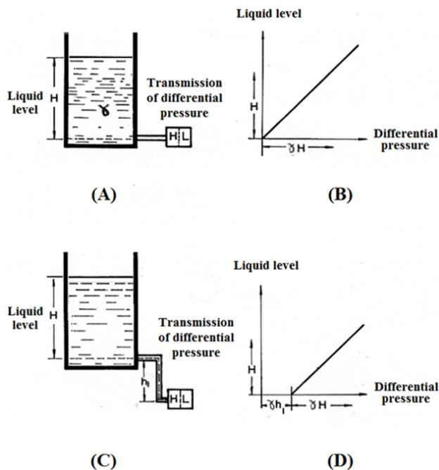
Fig. 5 Level measuring of the differential pressure type (open tank)
