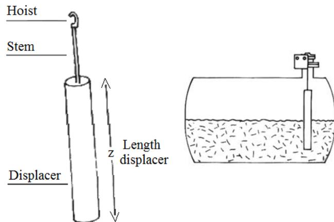
Fig. 1 Displacer typical
