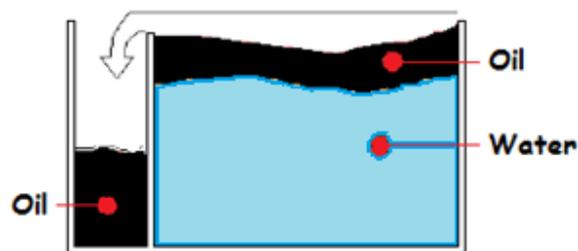
Fig. 3 Separator of oil and salt water
