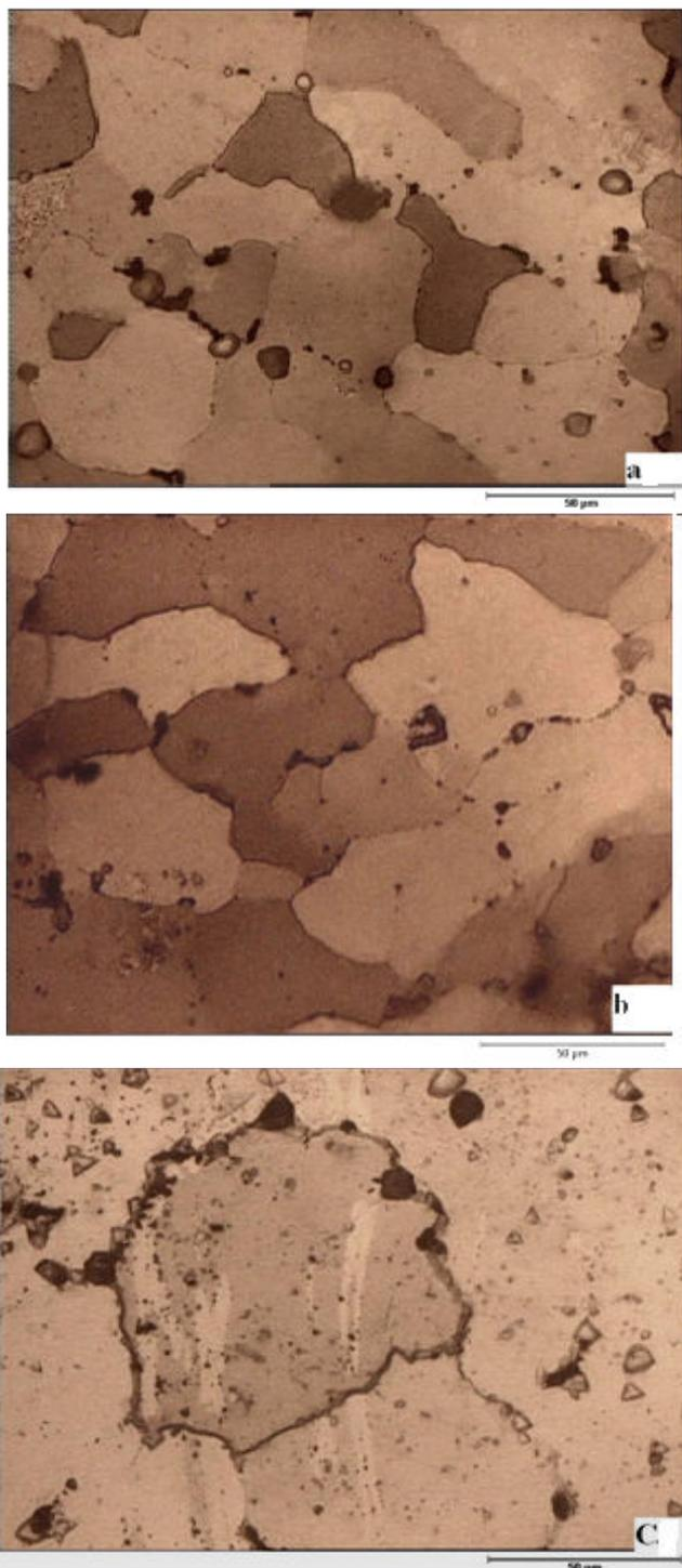
Fig. 5 Evolution of microstructure of 7055 Aluminum alloy with different reversion time: (a) 30 min; (b) 40 min; (c) 50 min.
