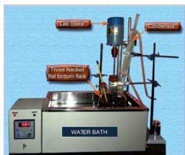
Fig. 1 Laboratory scale biodiesel reactor
