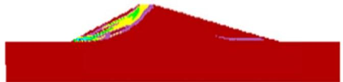
Fig. 5 Failure mechanism (shear deformations)
