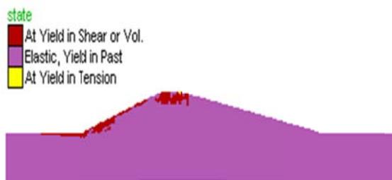
Fig. 8 Distribution of plasticity in the earth dam
