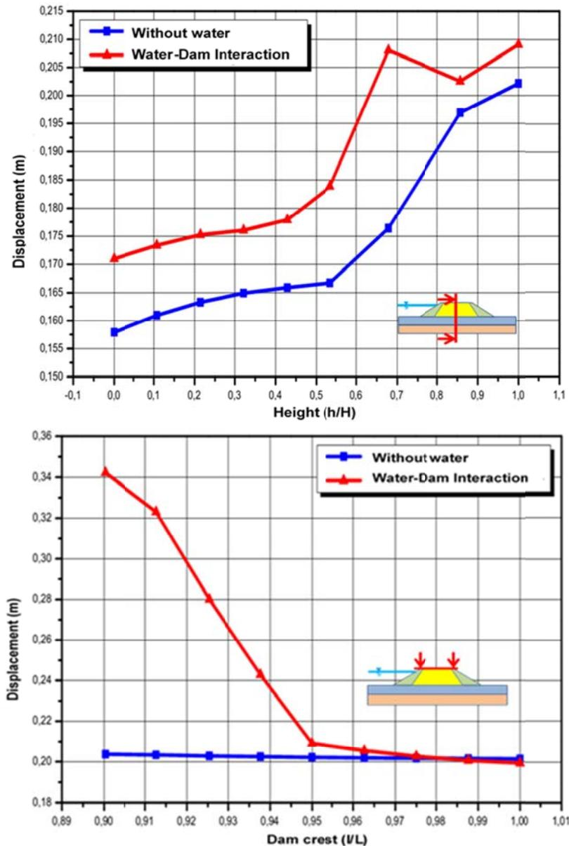
Fig. 7 Variation of the maximum horizontal displacement
