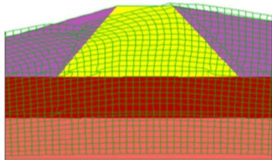
Fig. 4 Close-up view of the deformation of earth dam
