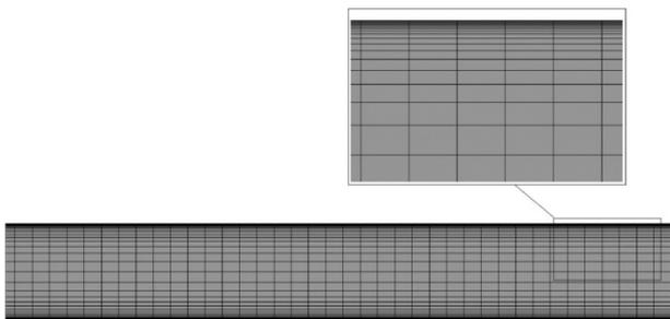
Fig. 4 Mesh configuration of annular channel
