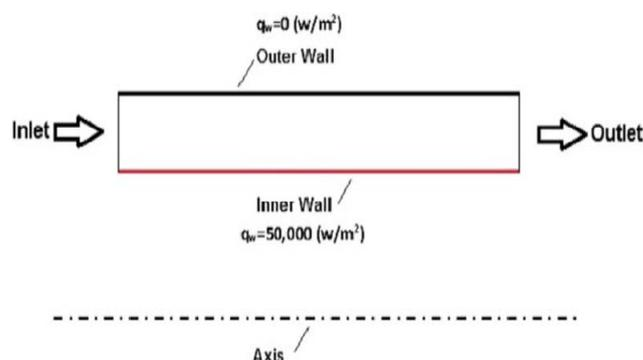
Fig. 1 2D geometrical configuration of annular channel
