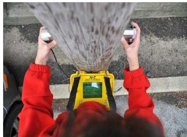
Fig. 6 UPV testing of concrete member
