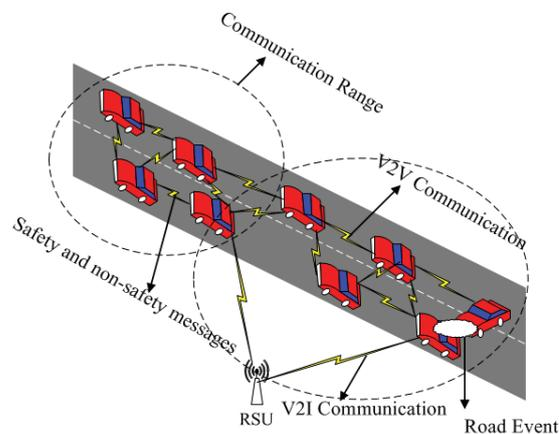
Fig. 1 VANET architecture represents V2V and V2I communication
