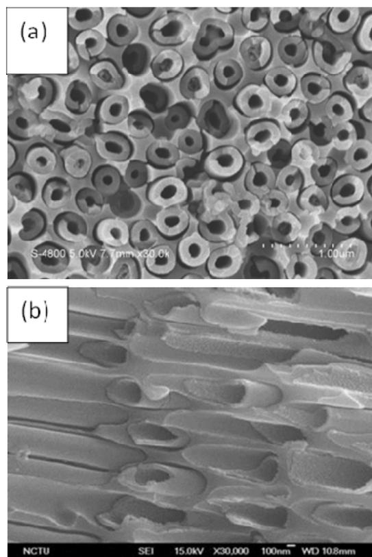
Fig. 4 SEM images of  $\text{TiO}_2$  NT in AAO template; (a) top view of  $\text{TiO}_2$  NT with 300 nm pore size on AAO template with 500 nm, (b) side view of  $\text{TiO}_2$  NTs inside AAO template
