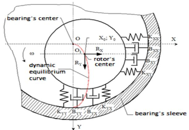
Fig. 6 Dynamic linearized model of the rotor system
