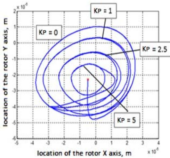
Fig. 4 Rotor's trajectory with various values of  $K_p$
