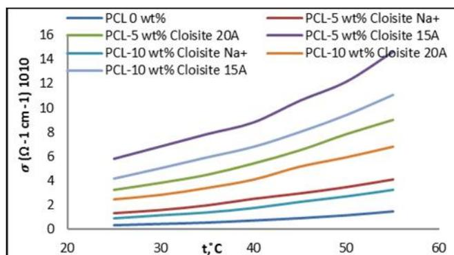
Fig. 18 Dependence of the electrical conductivity ( $\sigma$ ) on the temperature ( $t$ ) for PCL mixed with 5 and 10 wt% of Cloisite Na<sup>+</sup>, Cloisite 20A, and Cloisite 15A
