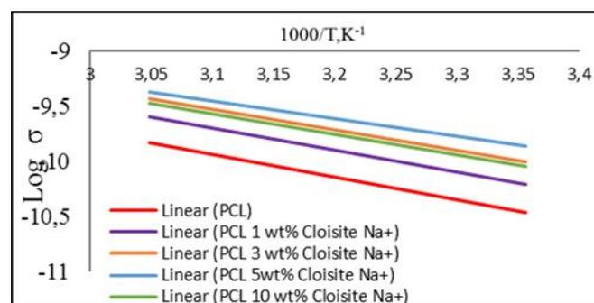
Fig. 19 Dependence of  $\log \sigma$  on  $10^3/T$  for PCL mixed with various proportions of Cloisite Na<sup>+</sup> (0, 1,3,5, and 10 wt%)
