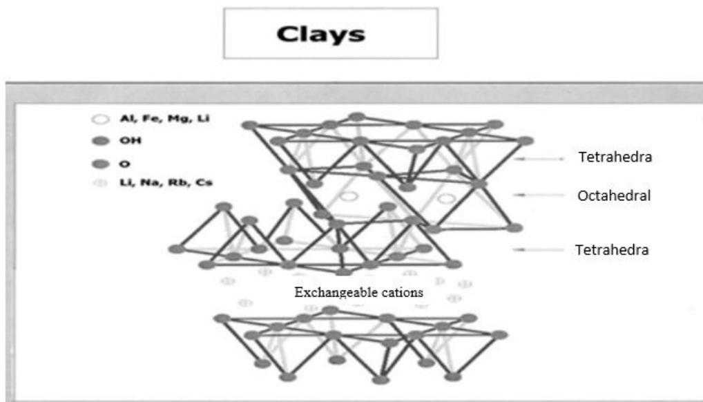
Fig. 1 The structure of a layered silicate [6]
