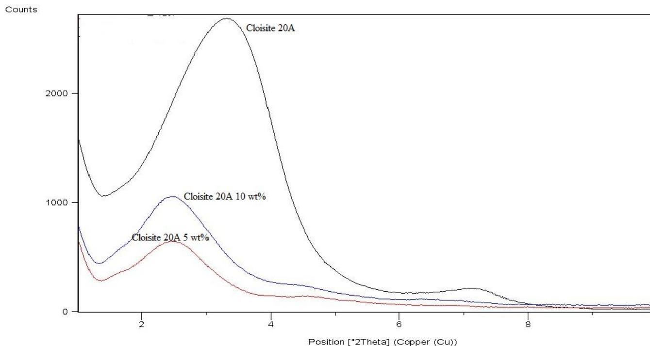
Fig. 22 XRD Patterns of Cloisite 20A and PCL/5 and 10 wt% Cloisite 20A nanocomposites
