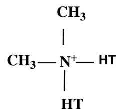
Fig. 3 Chemical modifier of Cloisites 20A and 15 A
