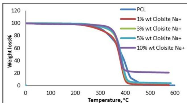
Fig. 7 TGA thermograms of PCL and PCL/1,3,5,10 wt% Cloisite Na<sup>+</sup> composites in air atmosphere
