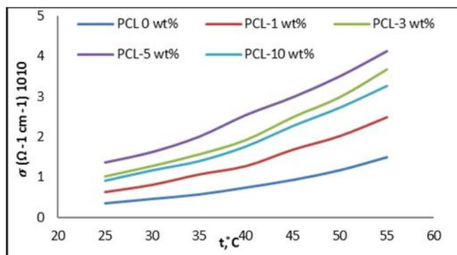
Fig. 17 Dependence of the electrical conductivity ( $\sigma$ ) on the temperature ( $t$ ) for PCL mixed with various proportions of Cloisite Na<sup>+</sup> (0,1,3,5, and 10 wt%)
