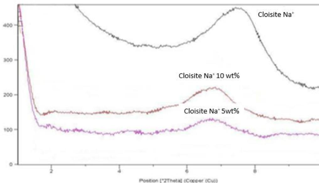
Fig. 21 XRD Patterns of Cloisite Na<sup>+</sup> and PCL/5 and 10 wt% Cloisite Na<sup>+</sup> composites
