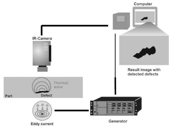
Fig. 2 Eddy current IR thermography – set-up
