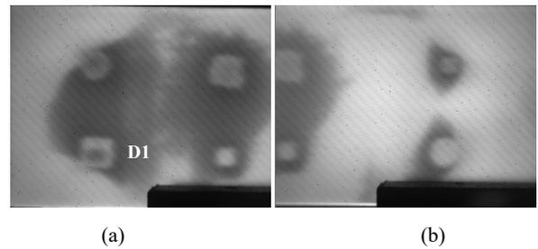
Fig. 6 The thermograms obtained by step heating method
