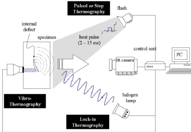
Fig. 1 IR thermography methods – set-up [6]
