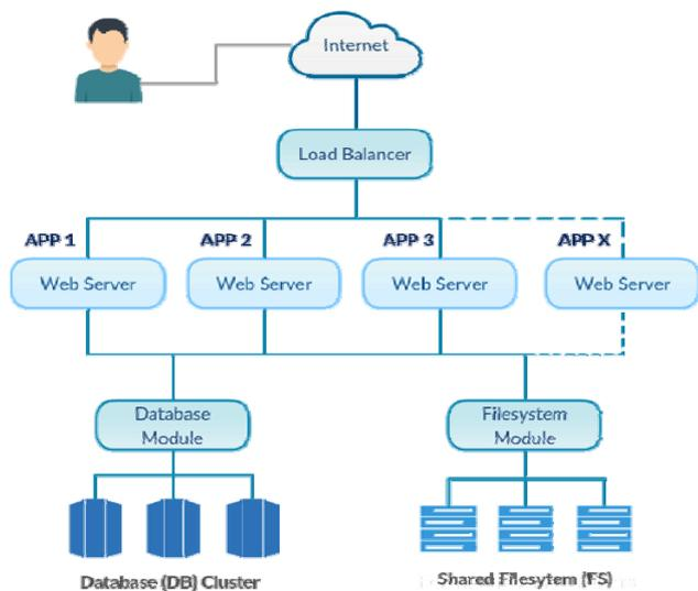
Fig. 3 Logic diagram of SCP's “scale-out” architecture
