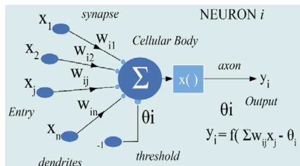
Fig. 2 Standard model of an artificial neuron [4]
