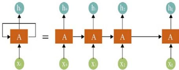
Fig. 6 Operation of a unit in an RNN [6]
