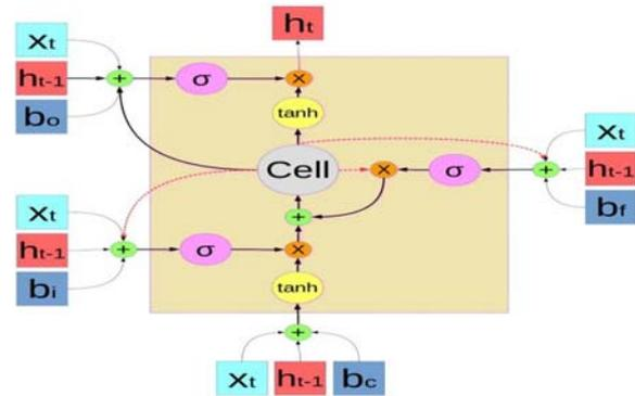
Fig. 8 Structure of a memory block [6]
