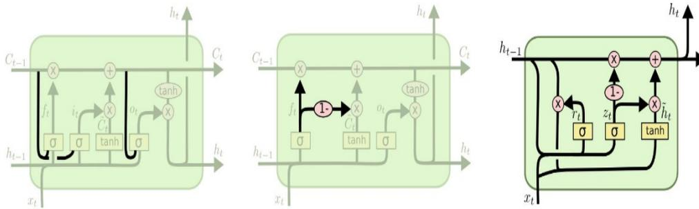
Fig. 10 Structure of a memory block [6]
