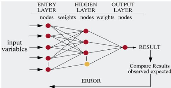
Fig. 3 Structure of a MLP [5]
