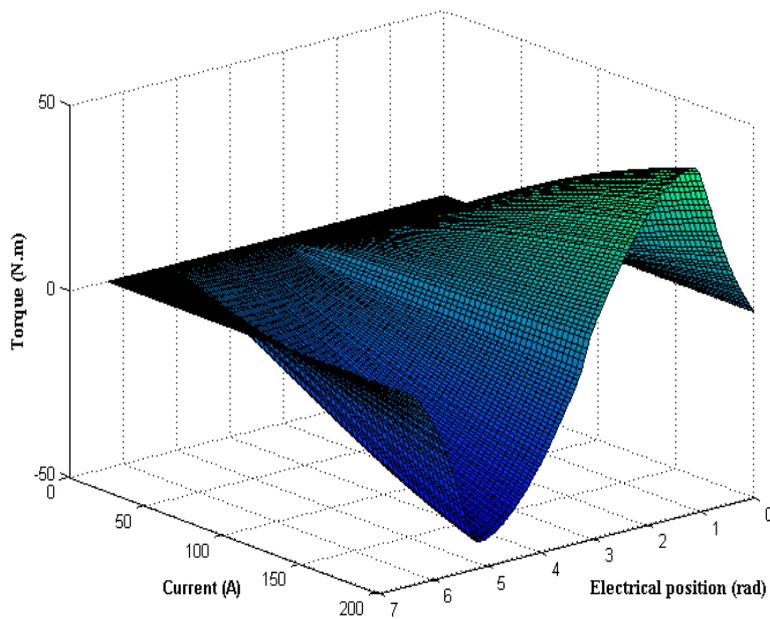
Fig. 3 3-D view of electromagnetic torque characteristic
