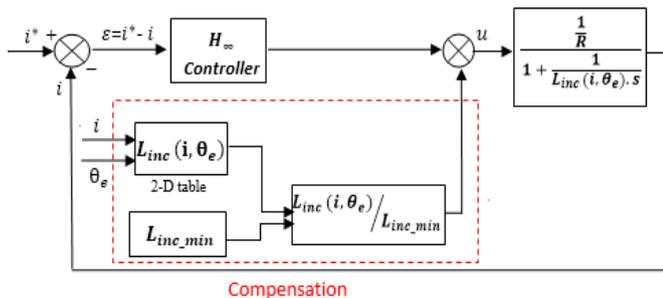
Fig. 6 Block diagram of the current loop
