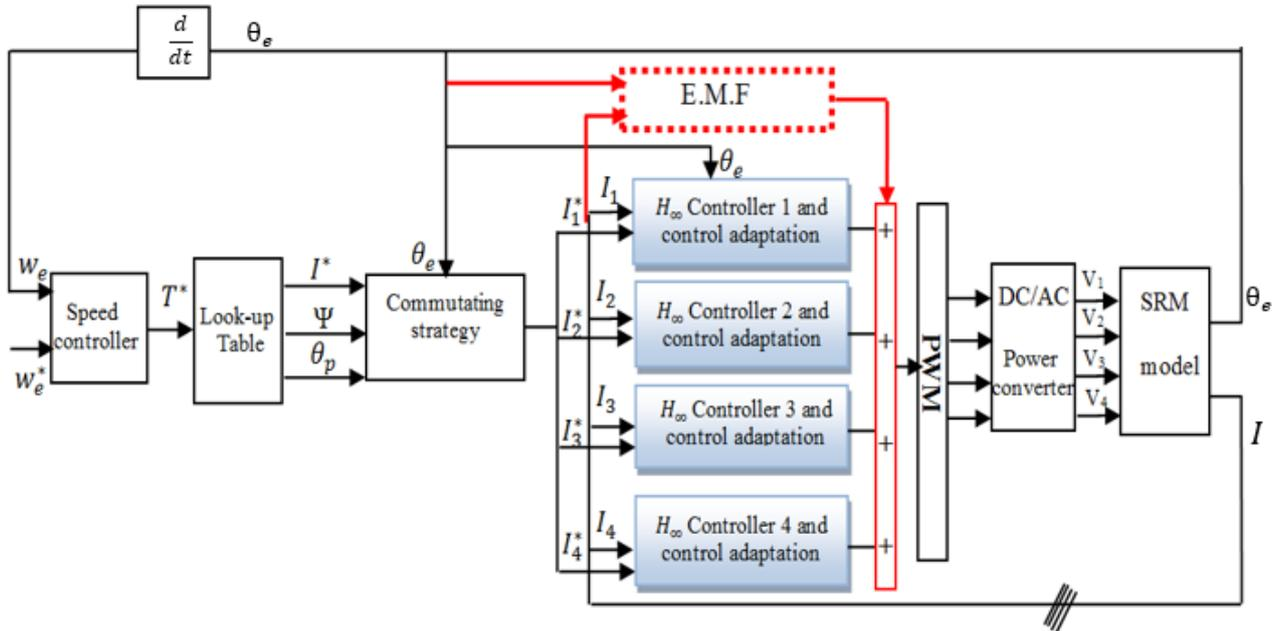
Fig. 5 Overall structure of the SRM control
