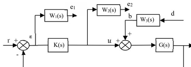
Fig. 4 Closed-loop scheme with the weighting transfer functions
