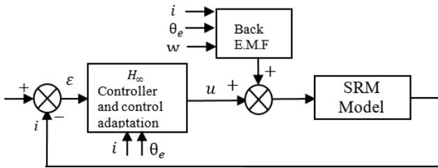
Fig. 8 Current control loop
