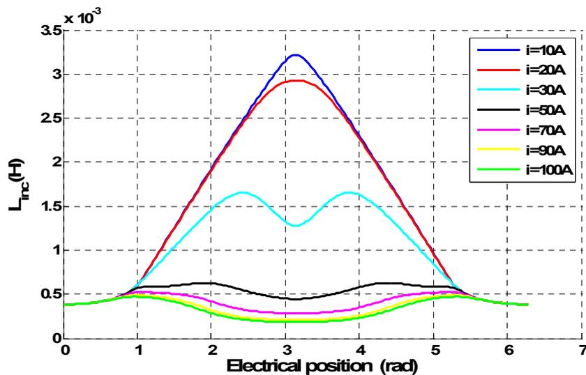
Fig. 1 Incremental inductance for one phase
