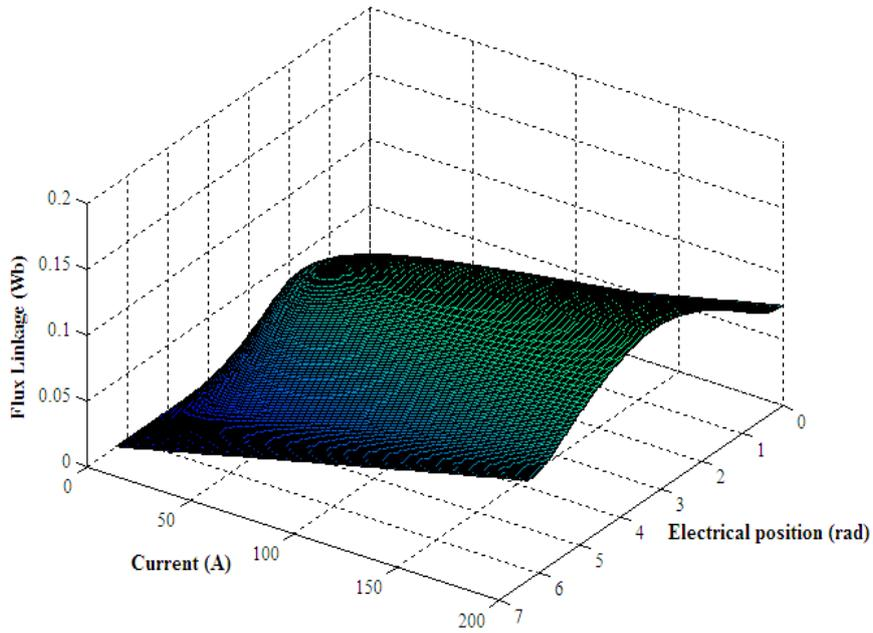
Fig. 2 3-D view of flux-linkage characteristic
