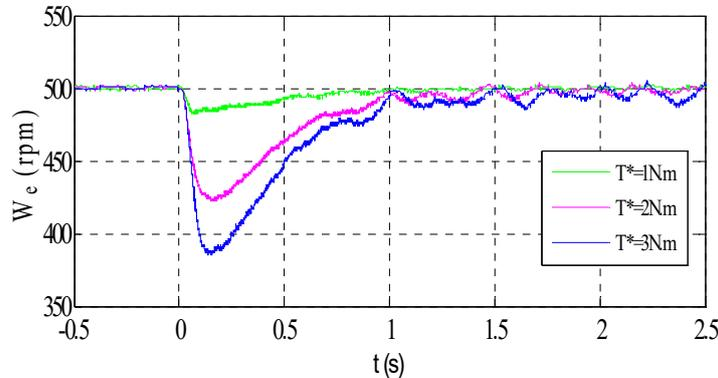
Fig. 15 Experimental speed responses; disturbance rejection at 500 rpm
