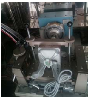
Fig. 4 Motor setting up using dynamo load tester in chamber
