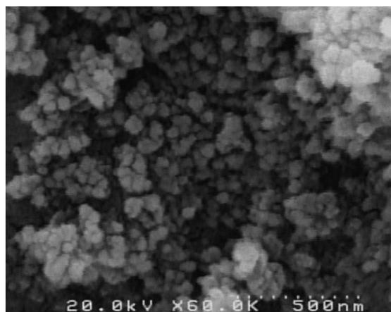
Fig. 1 SEM image of TiO<sub>2</sub> nanoparticles
