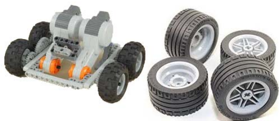
Fig. 2 Mindstorms NXT wheel-mounted motors
