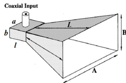
Fig. 2 Geometry of the proposed GPR horn antenna
