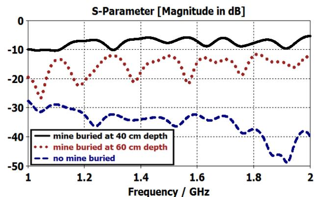
Fig. 6 Simulated  $S_{21}$  coefficient of landmine models for two different landmine burial depths (D)
