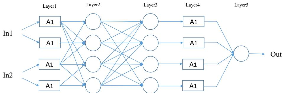
Fig. 2 Architecture of a typical ANFIS
