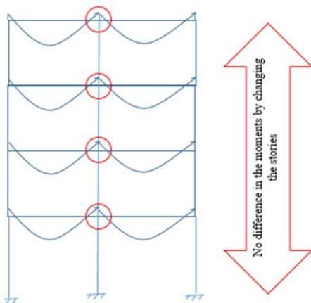
Fig. 3 The effect of height to the moments induced by gravitational loads
