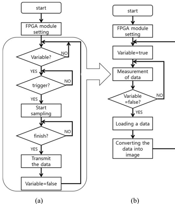
Fig. 2 Program flow chart (a) FPGA (b) Host
