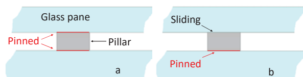
Fig. 3 Simulation conditions for support pillars: (a) top-bottom pinned pillars, and (b) bottom pinned-top sliding pillar
