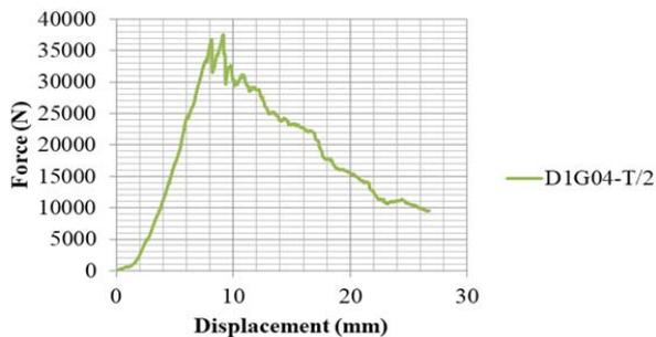
Fig. 19 Force-displacement diagram of the D1G04-T/2
