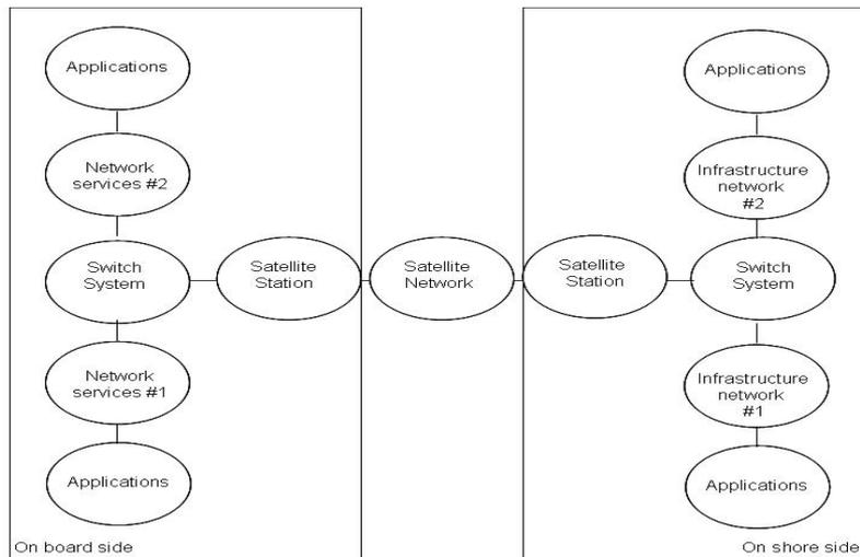
Fig. 9 Example of marine architecture with switch system
