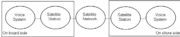
Fig. 5 Example of marine architecture without multiplexer
