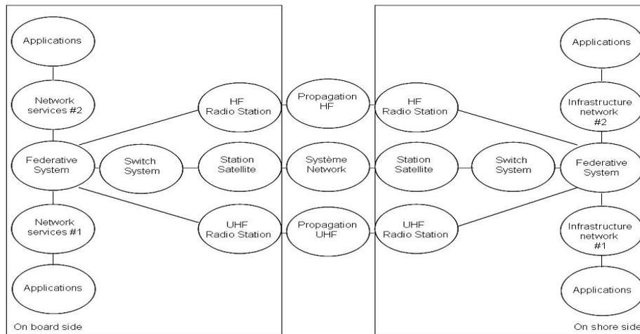
Fig. 13 Example of media switching marine architecture
