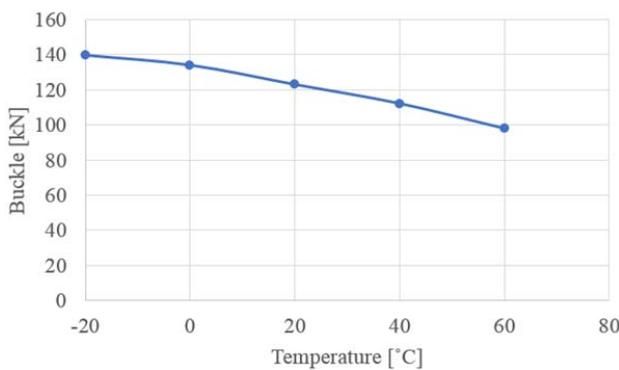
Fig. 4 Buckling load in term of temperature
