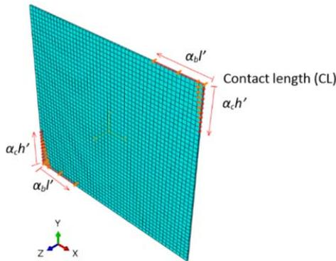
Fig. 2 FE model of PMC sandwich infill panel
