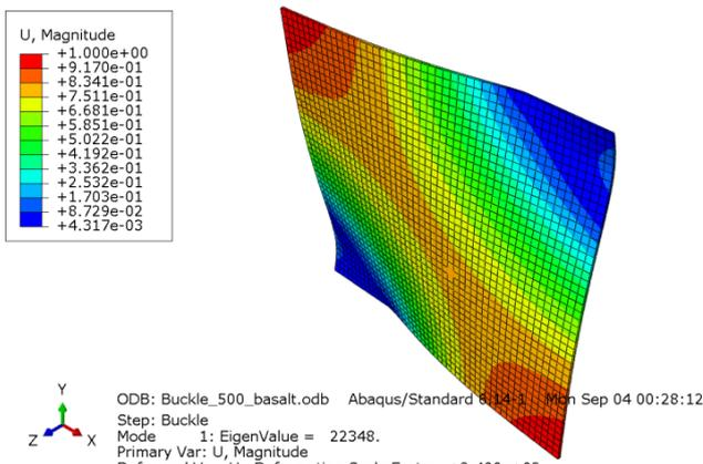
Fig. 3 Failure shape of infill panel system
