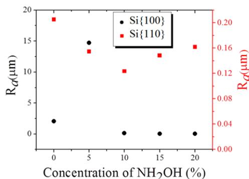
Fig. 4 Average surface roughness of Si{100} and Si{110} with varying concentrations of NH<sub>2</sub>OH (Etching time: 2 hr and etching temperature: 70±1°C; R<sub>a</sub> = Average surface roughness)
