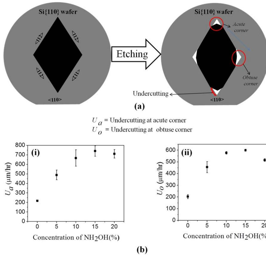
Fig. 3 Convex corner undercutting on Si{110} along <112> directions: (a) schematic view and (b) quantitative variation with varying concentrations of  $\text{NH}_2\text{OH}$  (Etching time: 1 hr and etching temperature:  $70 \pm 1^\circ\text{C}$ )
