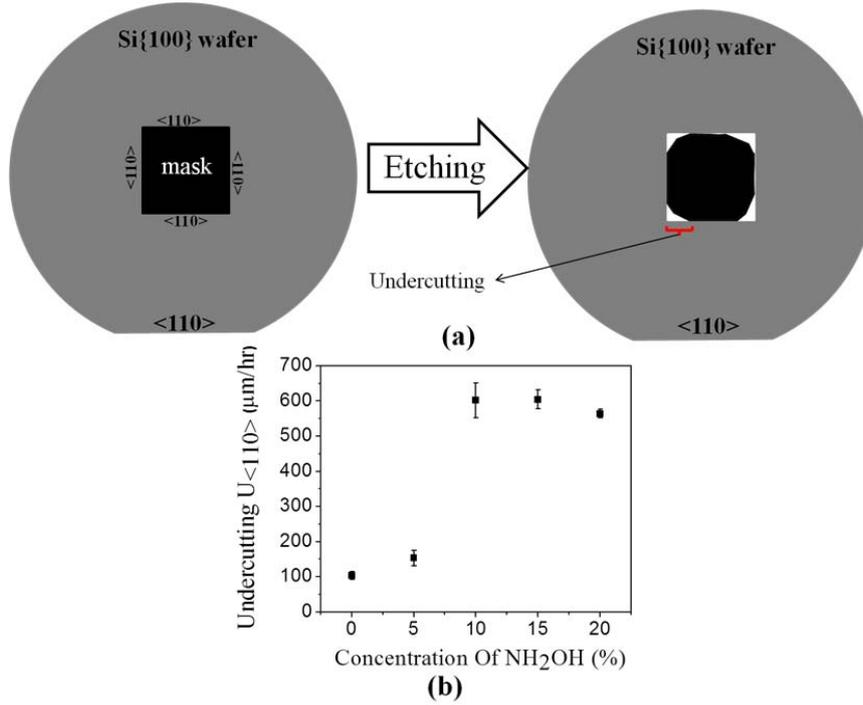
Fig. 2 Convex corner undercutting on Si{100} along <110> directions: (a) schematic view and (b) quantitative change with varying concentrations of  $\text{NH}_2\text{OH}$  (Etching time: 1 hr and etching temperature:  $70 \pm 1^\circ\text{C}$ )
