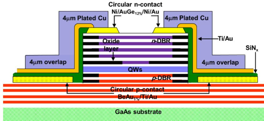
Fig. 1 A schematic cross-sectional view (not to scale) of the fabricated 850-nm VCSEL ready for testing
