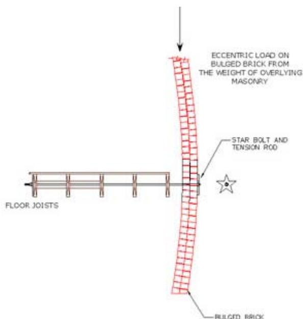
Fig. 4 Star bolt repair
