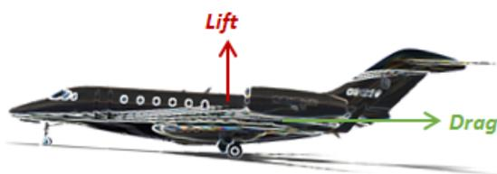
Fig. 1 Lift and drag forces applied on an aircraft
