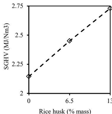
Fig. 4 Synthetic gas heating value for different blends
