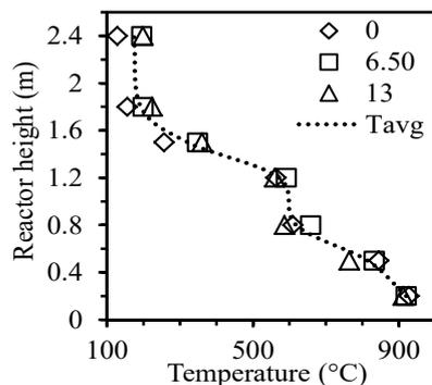
Fig. 2 Temperature profile along the height of reactor
