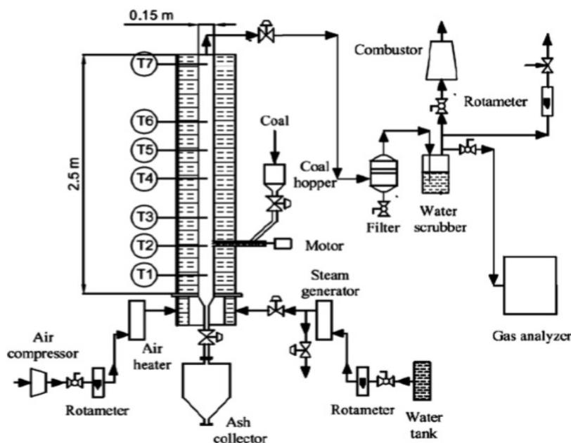
Fig. 1 Schematic of bubbling fluidized bed gasifier
