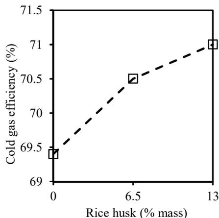
Fig. 5 Cold gas efficiency for different blends
