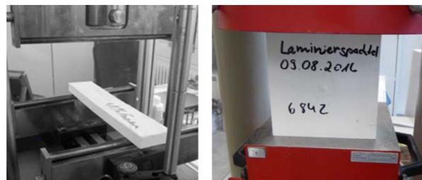
(a) Bending tensile strength (b) Compressive strength
