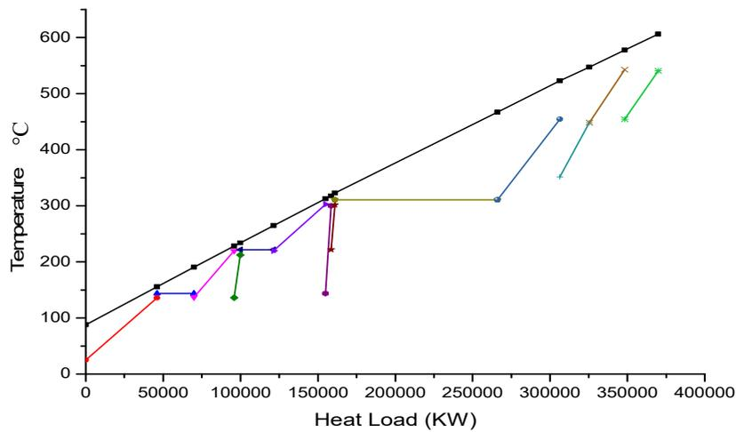
Fig. 3 Temperature-heat load (T-q) diagram in the HRSG of the NGCC
