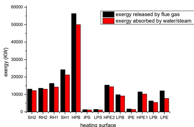
Fig. 17 Results of the exergy exchange in HRSG of the ISCC-DSG system with the replacement of HPE2+HPB+SH1
