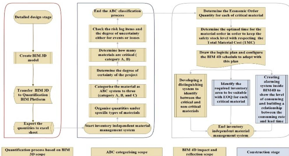
Fig. 4 BIM based material management automation (MaBIM) framework
