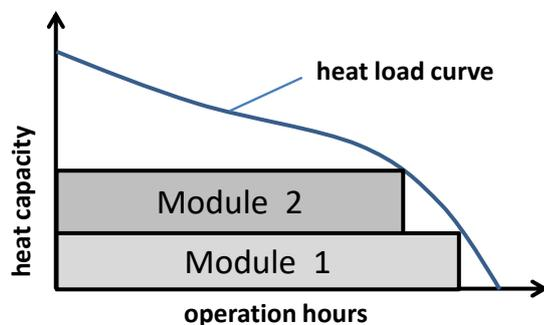
Fig. 7 Heat load curve with CHP modules
