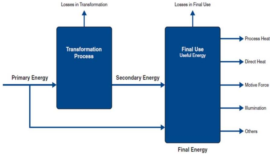
Fig. 1 Energy flow in an industrial plant [3]
