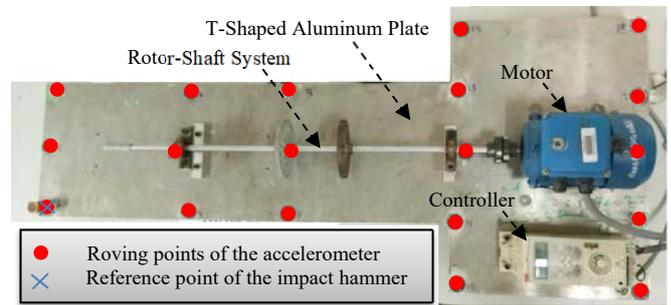
Fig. 2 Motor-driven test rig
