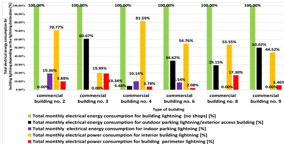
Fig. 3 (b) Total monthly electrical energy consumption for buildings lighting depending on lighting destination [%] - status for buildings with 8, 9, 10 operational years
