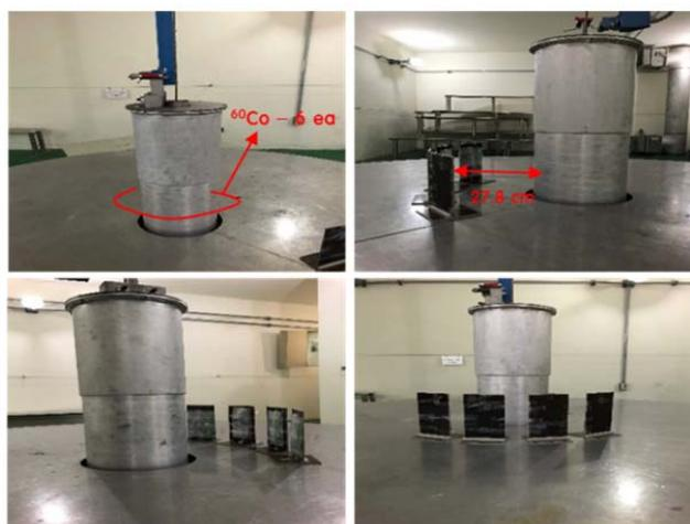
Fig. 2 Experimental set-up of gamma-ray irradiation of NPT-IGBTs
