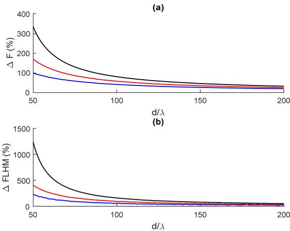
Fig. 3 (a) Focal displacement and (b)  $\Delta FLHM$  as a function of  $d$  for different focal distances:  $F = 15\lambda$  for blue solid line,  $F = 25\lambda$  for red solid line and  $F = 35\lambda$  for black solid line
