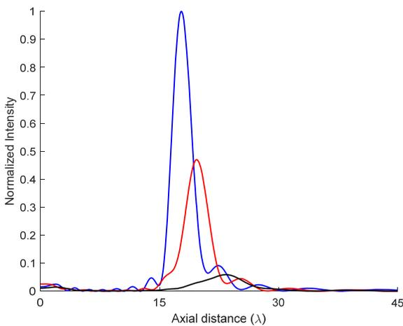
Fig. 7 Simulations for plane wave FZP design and piston emitter with  $ka = 15$ :  $d = 200\lambda$  for blue solid line,  $d = 120\lambda$  for red solid line and  $d = 60\lambda$  for black solid line
