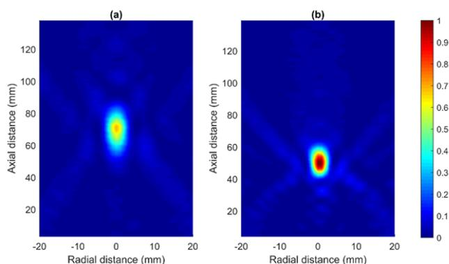
Fig. 9 Measured normalized intensity maps: (a) FZP design for plane wave incidence and (b) FZP design for spherical wave incidence
