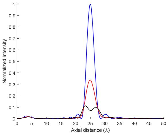
Fig. 6 Simulations for a FZP designed with spherical wave incidence consideration for different  $ka$  values:  $ka = 10$  for blue solid line,  $ka = 20$  for red solid line and  $ka = 30$  for black solid line
